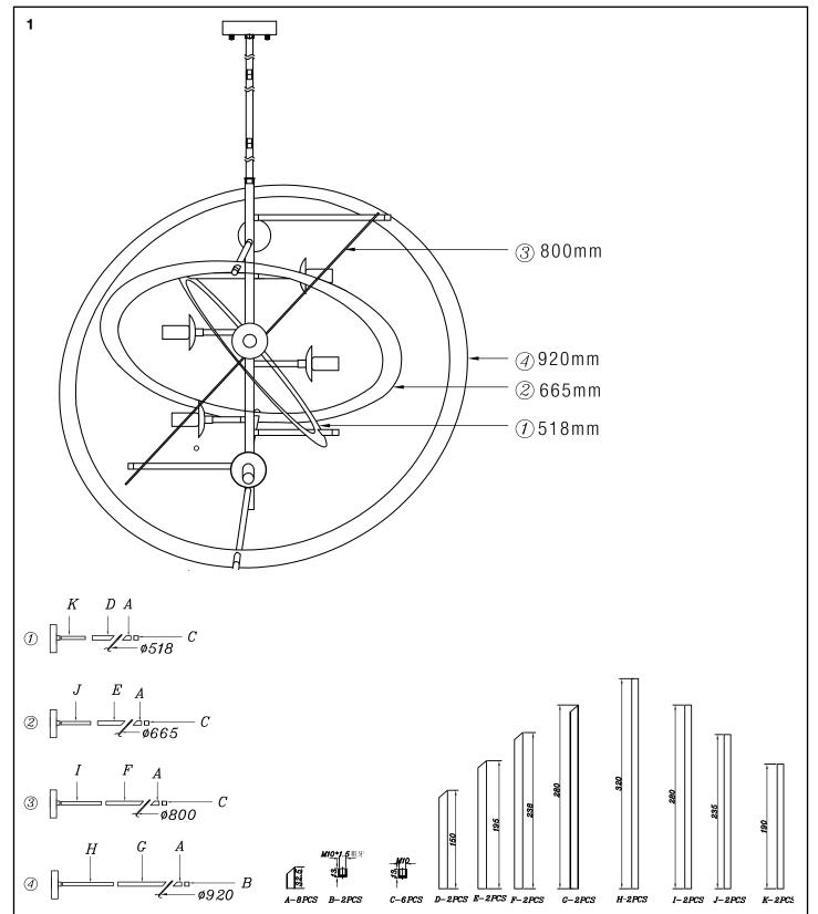
Fix the threaded rods (K) to the frame according to the drawing. Slide parts (D) over the rods. Place the 518mm ring over the rods. Slide tube (A) over the end of the rod and fix it with the nut (C).
