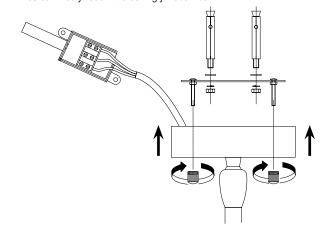
4 Connect the 3 power wires according to their colours. Brown is the live wire, blue is the neutral wire, green/yellow is the earth wire. Place the ceiling canopy (B) flush against the ceiling and fix it securely with the two nuts supplied.
