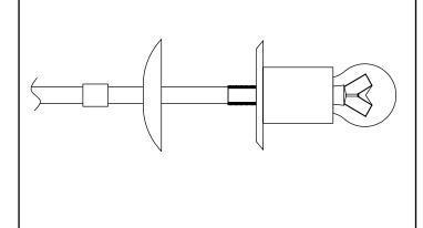
**7** Place the glass lampshade over the lampholder by tilting it around the gap in the plate and rotating it.
