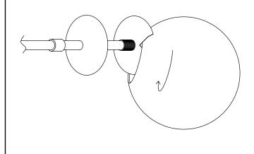
**8** Align the glass lampshade with the lamp holder. Fix the glass by tightening the nut.
