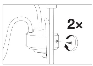
**3.** Place the lamp over the wall plate and align the holes in the lamp with the holes in the wall plate. Use an allen key to secure the screws on both sides of the lamp.
