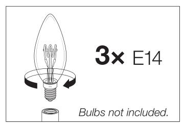
Carefully place the bulbs in the fittings. Do NOT turn the bulbs further than necessary, to prevent damage to the fitting.
