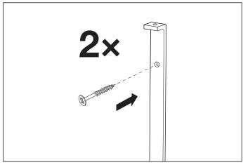
**2.** Fix the wall plate to the wall by using wall mounting plugs and screws suitable for your wall type.
