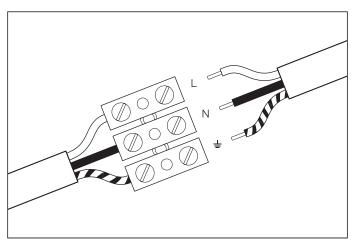
1. Connect the 3 wires according to their colours. Brown is the live wire, blue is the neutral wire, green/yellow is the earth wire.
