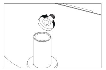
4. Tighten the knob until the lamp is secure.
