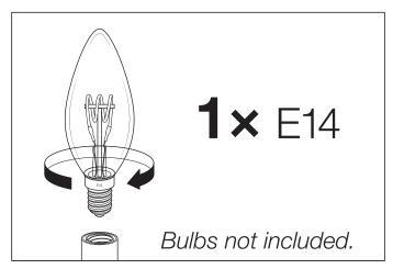
Carefully place the bulb in the fitting. Do NOT turn the bulb further than necessary, to prevent damage to the fitting.
