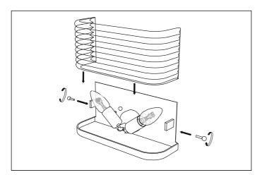
6. Place the glass and fix it with the knobs on the sides.
