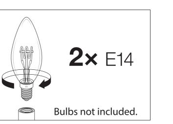
Carefully place the bulbs in the fittings. Do NOT turn the bulbs further than necessary, to prevent damage to the fitting.
