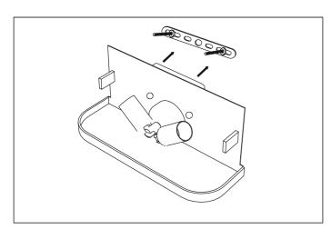
3. Place the lamp over the cross bar and fix it securely with the knobs.
