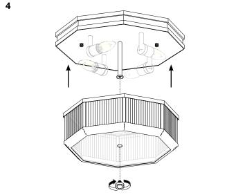
Turn off the electricity supply at the main circuit panel before installing. Do not connect the electricity supply until your luminaire is fully assembled and installed.
