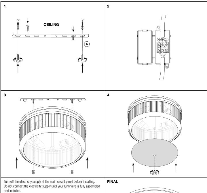
Fix the ceiling bracket (A) to the ceiling by using mounting plugs and screws suitable to your ceiling type.
