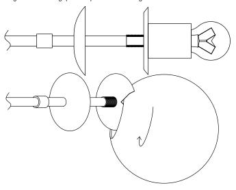
6 Align the glass lampshade with the lamp holder. Fix the glass by tightening the nut behind the plate.
