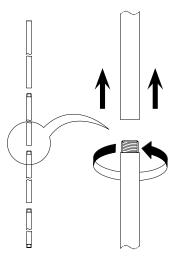
**2** Thread the wire from the lamp through the pipe.
