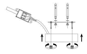
4 Connect the 3 power wires according to their colours. Brown is the live wire, blue is the neutral wire, green/yellow is the earth wire. Place the ceiling canopy flush against the ceiling and fix it securely with the two nuts supplied.
