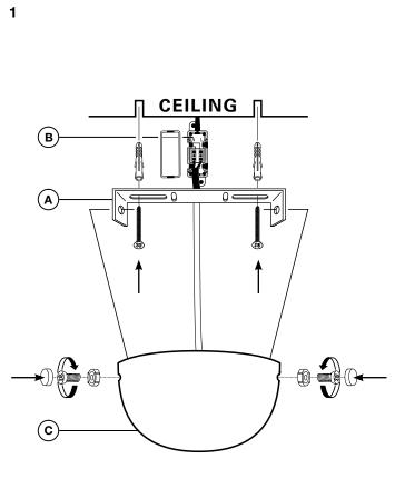
Turn-off the electricity supply at main circuit panel before installing. Do not connect electricity supply until your ceiling light is fully assembled and installed.
