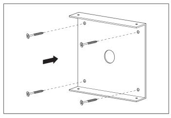
Fix the wall plate to the wall by using wall mounting plugs and screws suitable for your wall type.
