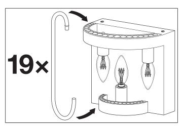
**5.** Carefully place the glass rods inside the holes on the frame. First place the bottom of the rod inside the hole, then the top side of the rod.
