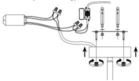
**5** Connect the 3 power wires with the transformer according to their colours. Brown is the live wire, blue is the neutral wire, green/yellow is the earth wire. Place the ceiling canopy flush against the ceiling and fix it securely with the two nuts supplied.
