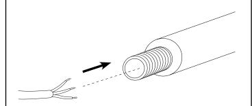
**4** Fix the ceiling plate (A) to the ceiling by using mounting plugs and screws suitable to your ceiling type. Guide the wires through the plate. Place or hold the lamp in an elevated position in such a way that the wires can freely reach the ceiling junction box.
