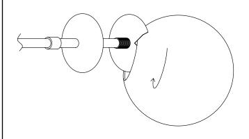
**8** Align the glass lampshade with the lamp holder. Fix the glass by tightening the nut.
