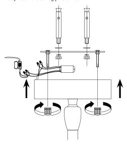
4 Connect the 3 power wires according to their colours to the connector. Brown is the live wire, blue is the neutral wire, green/yellow is the earth wire. Place the ceiling canopy (B) flush against the ceiling and fix it securely with the two nuts supplied.
