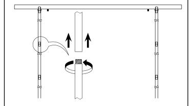
**4** Connect the 2 power wires to the transformer. Brown is the live wire, blue is the neutral wire. Slide the ceiling canopy over the ceiling plate and and fix it securely with the two nuts supplied.
