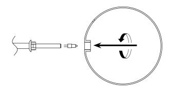
**3** Fix the ceiling plate to the ceiling by using mounting plugs and screws suitable to your ceiling type. Guide the wires through the plate. Place or hold the lamp in an elevated position in such a way that the wires can freely reach the ceiling junction box.
