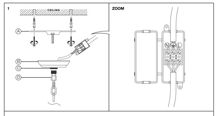
Turn off the electricity supply at the main circuit panel before installing. Do not connect the electricity supply until your luminaire is fully assembled and installed.
