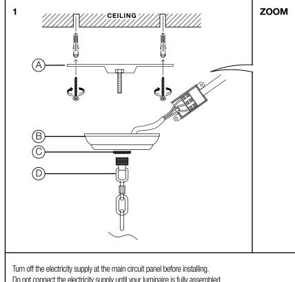
Do not connect the electricity supply until your luminaire is fully assembled and installed.
