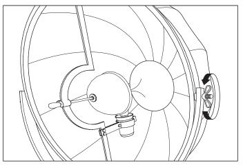
**4.** To adjust the position of the shade loosen the wing nuts on the sides and tighten them to secure it in the desired position.
