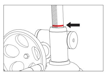
**6.** Do NOT turn the wheel beyond the red mark on the centre pipe to avoid damage to the mechanism.
