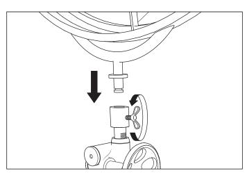
3. Loosen the knob and place the lamp on the stand, tighten the knob to secure it.
