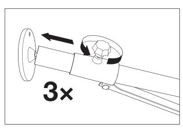
Loosen all three knobs by turning them anti-clockwise. Extend the legs one by one and tighten the knobs until the legs are secure.
