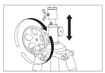
5. To change the height of the lamp, turn the wheel clockwise.
