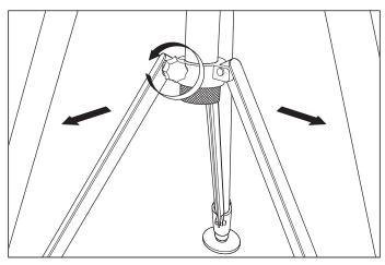
2. Loosen the centre knob and tighten it after placing the stand upright.
