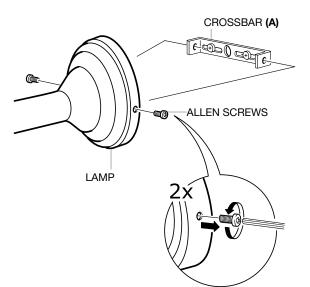
Turn off the electricity supply at the main circuit panel befor installing. Do not connect the electricity sypply until your luminaire is fully assembled and installed.
