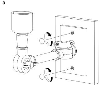
Turn off the electricity supply at the main circuit panel before installing. Do not connect the electricity supply until your luminaire is fully assembled and installed.
