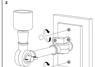
Turn off the electricity supply at the main circuit panel before installing. Do not connect the electricity supply until your luminaire is fully assembled and installed.
