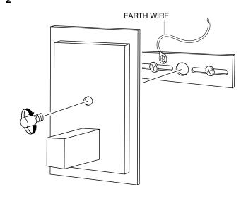
Turn-off the electricity supply at the main circuit panel before installing. Do not connect electricity supply until your wall lamp is fully assembled and installed.
