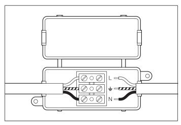
2. Connect the 3 wires according to their colours. Brown is the live wire, blue is the neutral wire, green/yellow is the earth wire.
