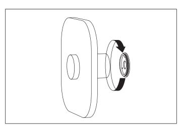
3. Screw the lamp on the wall plate.
