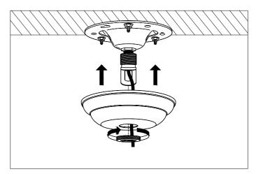
2. Slide the canopy over the ceiling bracket and fix it with the retaining nut.
