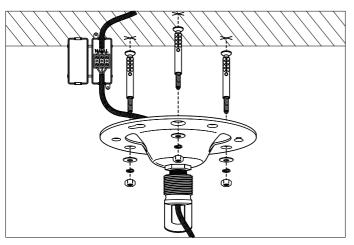
Fix the ceiling bracket to the ceiling by using mounting plugs and screws suitable for your ceiling type. Connect the 3 power wires. Brown is the live wire, blue is the neutral wire, green/yellow is the earth wire.
