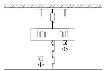
**3.** Carefully place the canopy over the ceiling plate and fix the canopy with the nuts provided.
