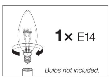
Carefully place the bulb in the fitting. Do NOT turn the bulb further than necessary, to prevent damage to the fitting.
