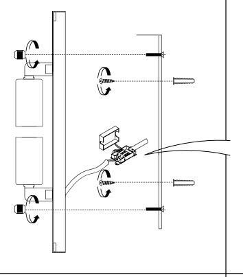
**2** Connect the 3 wires according to their colours. Brown is the live wire, blue is the neutral wire, green/yellow is the earth wire.
