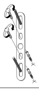
2 Connect the 3 wires according to their colours. Brown is the live wire, blue is the neutral wire, green/yellow is the earth wire.
