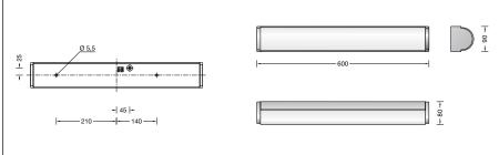
Luminaire with lampholder E 14 Lamp wattage max. 4 × 40 W
