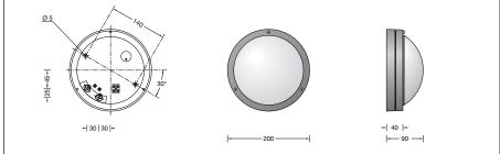
Luminaire with lampholder E 14 Lamp output max. 60 W
