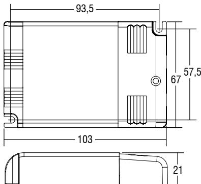
**BUILT-IN** **SCREW FIXING** Weight - Peso gr. 120
