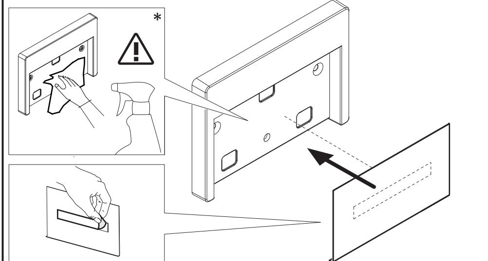
\* CLEAN THE FIXING SURFACE WITH ALCOHOL OR SOLVENT BEFORE GLUING THE PLATE
