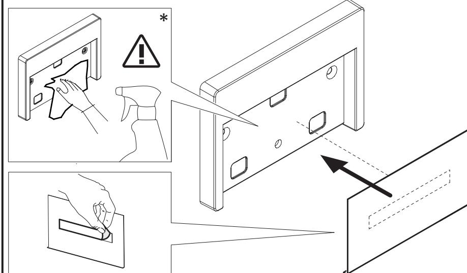
\* CLEAN THE FIXING SURFACE WITH ALCOHOL OR SOLVENT BEFORE GLUING THE PLATE
