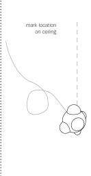
Move pendant into location and mark the location for the swag hook screw on the ceiling.
