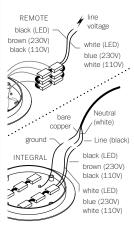
Connect transformers inside the canopy to line voltage.
