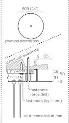
2 Note: The client is responsible for providing a robust 19mm (3/4") plywood backing or wood blocking to securely anchor to
