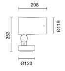
Spotlight with base - Warm White Led - integrated electronic control gear - Wide Flood optic Photometric data for this product will be available starting from June 2018.
