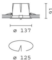
**recessed luminaire Ø 137 - warm white passive dissipation LED - CRI (Ra) > 90 - integrated DALI control gear - flood****Product code**
