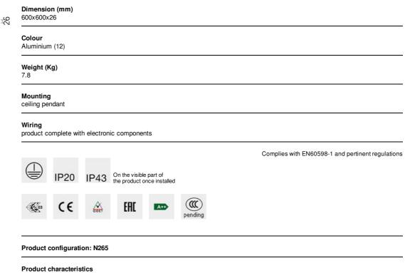
Total lighting output [Lm]: 4209 Total power [W]: 41.8 Luminous efficacy [Lm/W]: 100.7 Life Time: > 50,000h - L80 - B10 (Ta 25°C)
