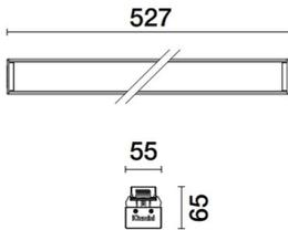
**Grazing effect light module - L 528 - warm LED - DALI control gear - wall washer**
