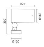
Spotlight with base - Neutral White Led - integrated electronic control gear - Medium optic etric data for this product will be available starting from September 2018
