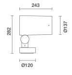
Spotlight with base - Neutral White Led - integrated electronic control gear - Spot optic etric data for this product will be available starting from September 2018
