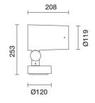
Spotlight with base - Warm White Led - integrated electronic control gear - Medium optic
