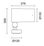
Spotlight with base - Warm White Led - integrated electronic control gear - Spot optic Photometric data for this product will be available starting from September 2018.
