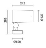
Spotlight with base - Warm White Led - integrated electronic control gear - Spot optic etric data for this product will be available starting from Septe
