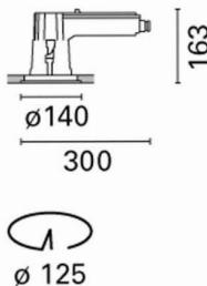
**Ceiling-mounted recessed luminaire with IP66 protection rating, small body with box, Warm White COB LEDs, fixed Flood Optic - Dimm. DALI**
