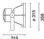
**Spotlight with bracket - Warm White COB LED - Integrated dimm electronic control gear DALI - Wide Flood optic**
