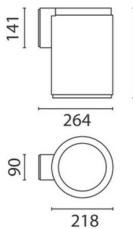
**Outdoor wall-mounted luminaire - warm white LED - with integrated electronic ballast Vin=120-277V ac - Wide Flood optic****Product code**
