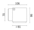
Outdoor wall-mounted luminaire - Neutral white LED - with electronic ballast Vin=100-240V ac - Flood optic
