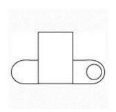
Flush double-projector pole top, attachment 120 mm -
