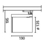
Sydecar - with electronic control gear 150W HIT (CDM-T) - Spot
