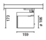
Sydecar - with electronic control gear 35W HIT (CDM-TC) - Flood
