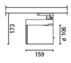
Sydecar - with dimmable electronic transformer 100W 12V QT 12 - Flood
